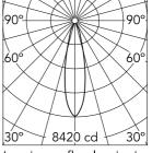
Luminous flux luminaire 1855 lm
