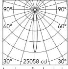
Luminous flux luminaire 1945 lm
