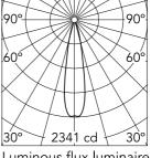
Luminous flux luminaire 412 lm (EXTREME CUT OFF)
