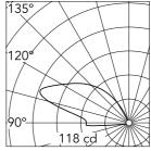
Luminous flux luminaire 621 lm
