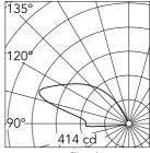
Luminous flux luminaire 2173 lm
