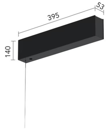
Surface power supply with driver included 320W / 48Vdc. 1-10V / 0-10V / No dim.
