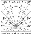
Luminous flux luminaire 1688 lm
