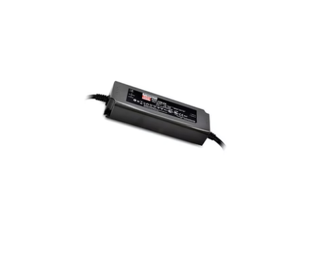
Electronic transformer with constant voltage (24V) for LED. 100/240V. 120W 60.9407
