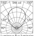
Luminous flux luminaire 1266 lm
