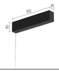
Surface power supply for direct and indirect lighting with housing for the driver 08.8886.14
