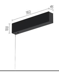
DALI controller and 24V/185W equipment to supply and control both the direct and indirect lighting, included 08.8886.14.DA
