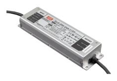
LED power supply source for remote installation in 24V/200W electric control panel. To avoid problems of overload it is recommended to install a power source every 185W. 100/240V. 60.9352
