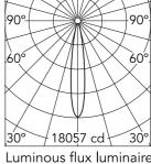
Beam Angle: 16° h(m) = E(Ix)D(m) 18057 0.28 4514 0.56 3 2006 0.84 1129 1.12 5 722 1.40
