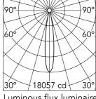
Luminous flux luminaire 1951 lm
