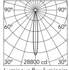
Luminous flux luminaire 1553 lm (EXTREME CUT OFF)
