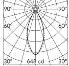
Luminous flux luminaire 313 lm (EXTREME CUT OFF)
