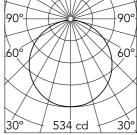
Luminous flux luminaire 1529 lm
