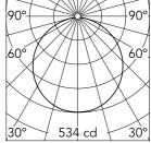
Luminous flux luminaire 1529 lm
