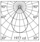
Luminous flux luminaire 1982 lm
