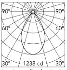
Luminous flux luminaire 1171 lm
