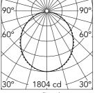
Luminous flux luminaire 4802 lm (EXTREME CUT OFF)
