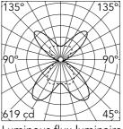
Luminous flux luminaire 3547 lm (EXTREME CUT OFF)
