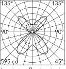
Luminous flux luminaire 3408 lm (EXTREME CUT OFF)
