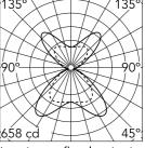
Luminous flux luminaire 4398 lm (EXTREME CUT OFF)
