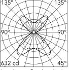
Luminous flux luminaire 4225 lm (EXTREME CUT OFF)
