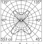
Luminous flux luminaire 3526 lm (EXTREME CUT OFF)
