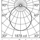
Luminous flux luminaire 4998 lm (EXTREME CUT OFF)
