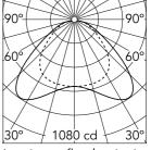
Luminous flux luminaire 3775 lm (EXTREME CUT OFF)
