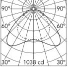
Luminous flux luminaire 3627 lm (EXTREME CUT OFF)
