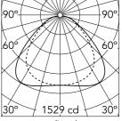
Luminous flux luminaire 4441 lm (EXTREME CUT OFF)
