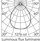
88° Beam Angle: h(m) = E(Ix)D(m) 1276 1.99 2 319 3.98 3 142 5.97 80 7.97 51 9.96
