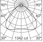
Luminous flux luminaire 3919 lm (EXTREME CUT OFF)
