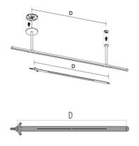
Aluminium Stencil Installation. D: 1100mm 08.0032.00
