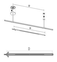
Aluminium Stencil Installation. D: 1600mm 08.0033.00
