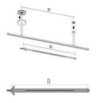
Aluminium Stencil Installation. D: 1100mm 08.0032.00
