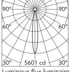
4 350 30° 5601 cd 30° 5 224 Luminous flux luminaire 428 lm
