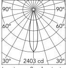
Luminous flux luminaire 406 lm (EXTREME CUT OFF)
