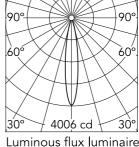
Luminous flux luminaire 505 lm
