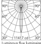
Luminous flux luminaire 539 lm (EXTREME CUT OFF)
