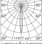
Luminous flux luminaire 539 lm
