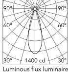
32° Beam Angle: h(m) = E(Ix)D(m) 1400 0.58 2 1.16 350 3 156 1.75 4 88 2.33 5 56 2.91
