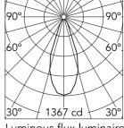
Beam Angle: 40° h(m) = E(Ix)D(m) 1367 0.73 2 342 1.45 3 152 2.18 4 2.91 85 55 3.64
