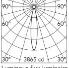
Luminous flux luminaire 487 lm
