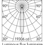
Luminous flux luminaire 2845 lm
