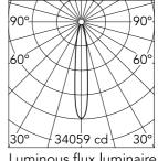
Luminous flux luminaire 5003 lm
