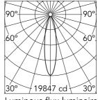
Luminous flux luminaire 4655 lm
