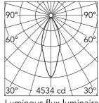
Luminous flux luminaire 1772 lm
