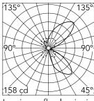
Luminous flux luminaire 2200 lm
