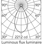
51° Beam Angle: h(m) = E(Ix)D(m) 2212 0.95 2 1.90 553 3 246 2.85 4 138 3.79 5 88 4.74
