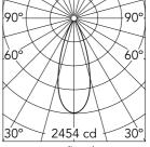
Luminous flux luminaire 1043 lm
