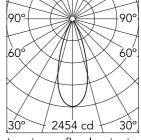
Luminous flux luminaire 1043 lm
